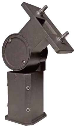
ADJUSTABLE SLIP FITTER MOUNT (WILL MOUNT TO 2" PIPE, 2.38" O.D.) 6 LBS. / EPA .3355 SQ. FT.
